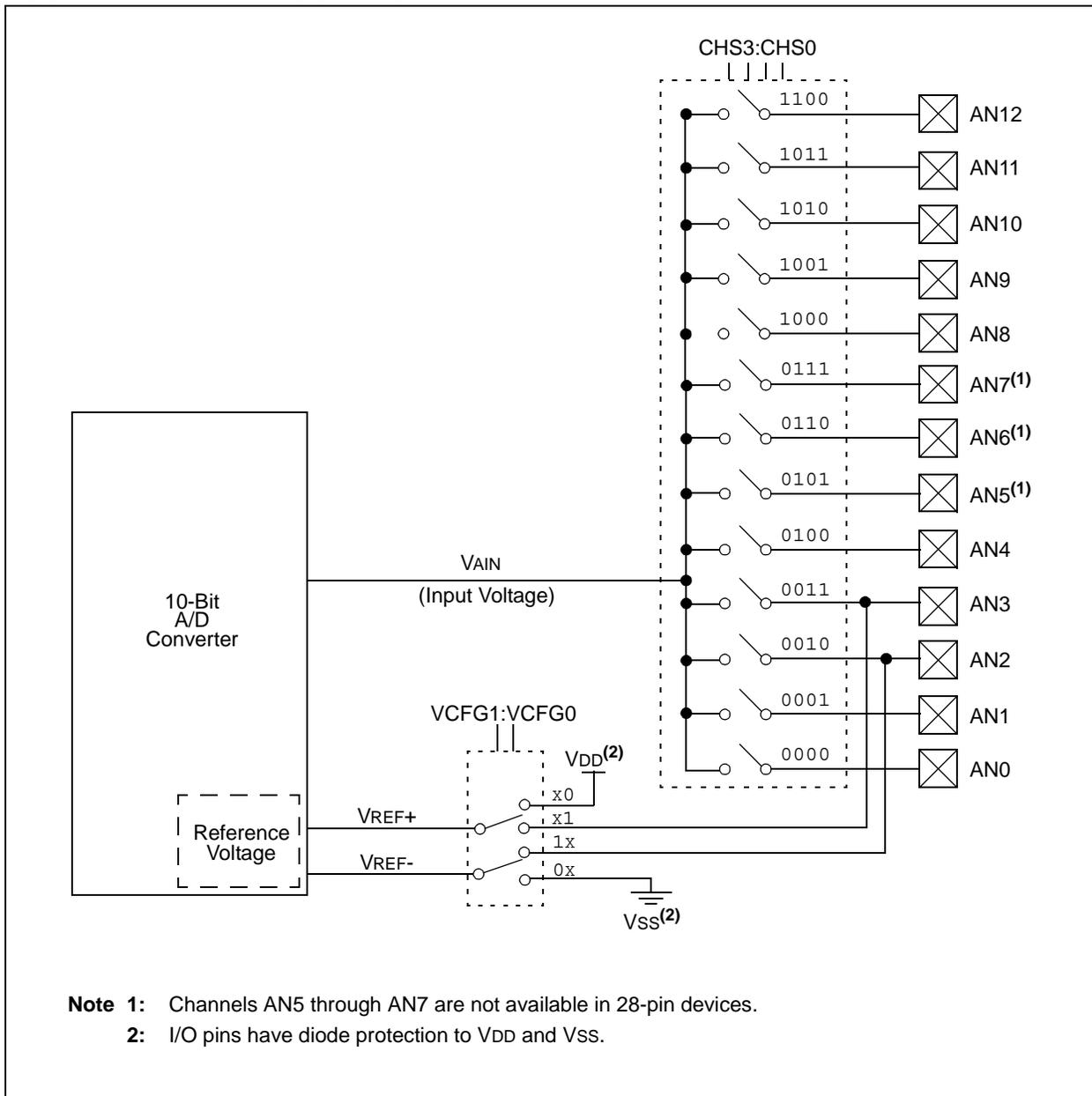
After the A/D module has been configured as desired, the selected channel must be acquired before the conversion is started. The analog input channels must
