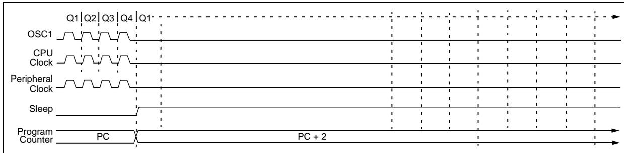
**FIGURE 3-5: TRANSITION TIMING FOR WAKE FROM SLEEP**
