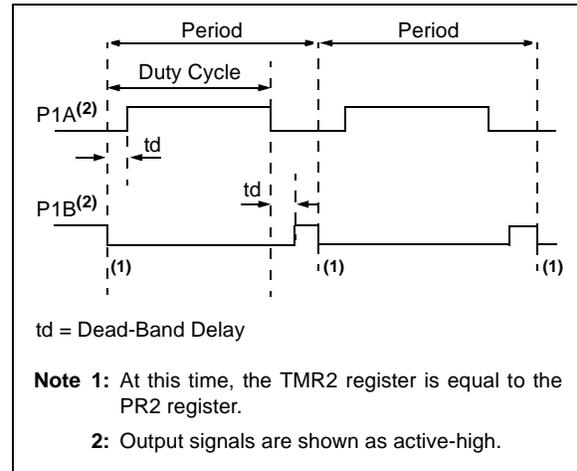
**FIGURE 14-5: EXAMPLES OF HALF-BRIDGE OUTPUT MODE APPLICATIONS**
