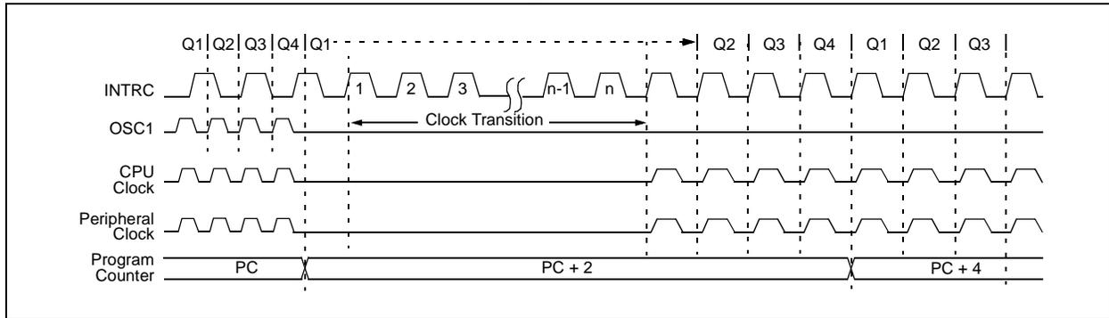
**FIGURE 3-3: TRANSITION TIMING FROM RC\_RUN MODE TO PRI\_RUN MODE**
