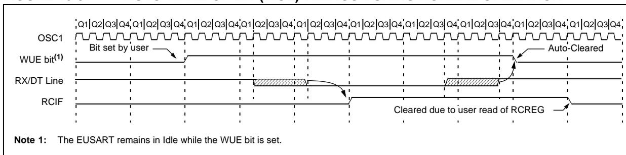
**FIGURE 16-9: AUTO-WAKE-UP BIT (WUE) TIMINGS DURING SLEEP**
