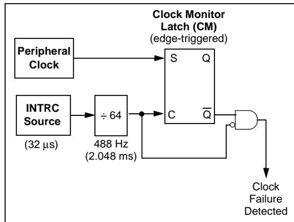
Clock failure is tested for on the falling edge of the sample clock. If a sample clock falling edge occurs while CM is still set, a clock failure has been detected (Figure 20-5). This causes the following:
