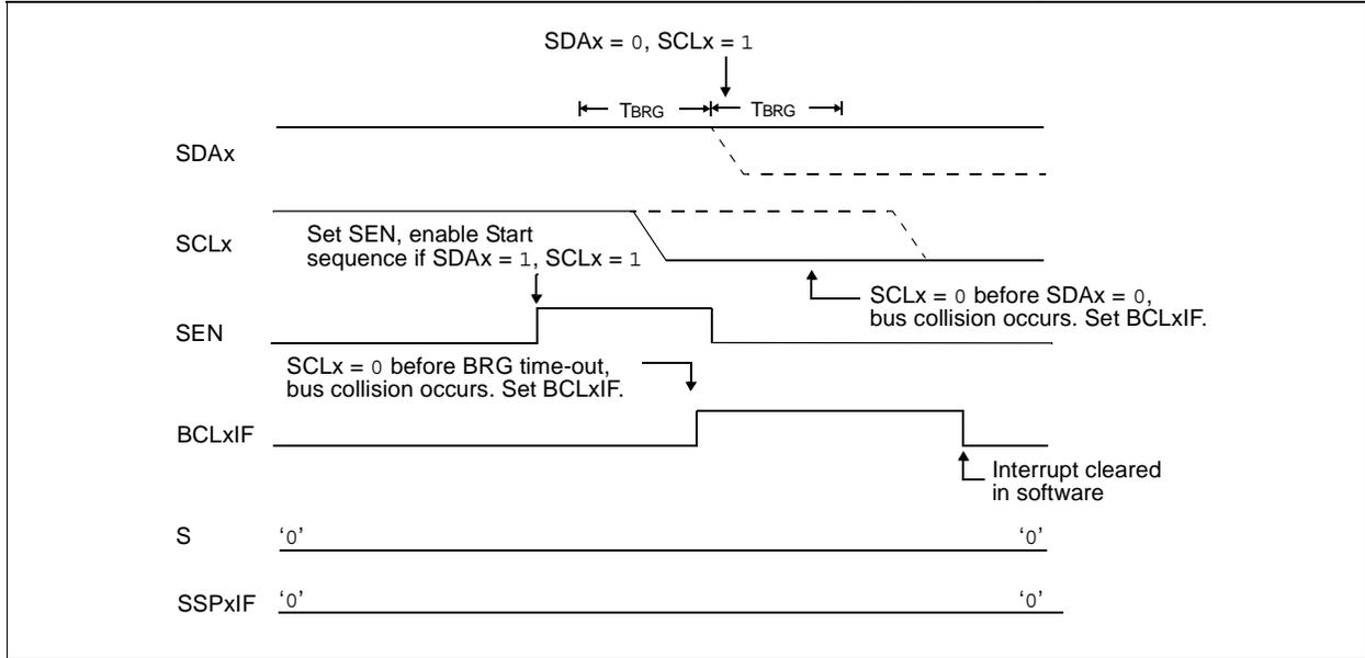
**FIGURE 15-28: BRG RESET DUE TO SDAx ARBITRATION DURING START CONDITION**
