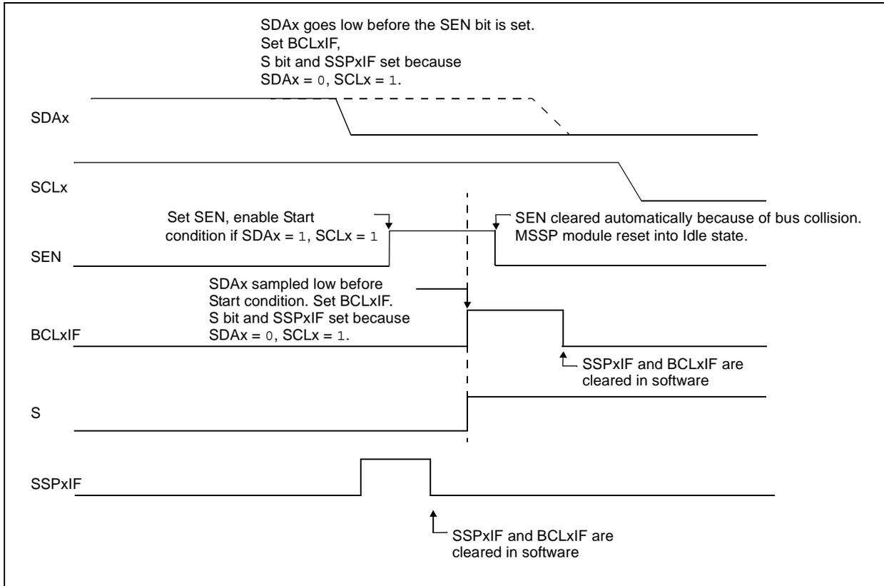
**FIGURE 15-27: BUS COLLISION DURING START CONDITION (SCLx = 0)**
