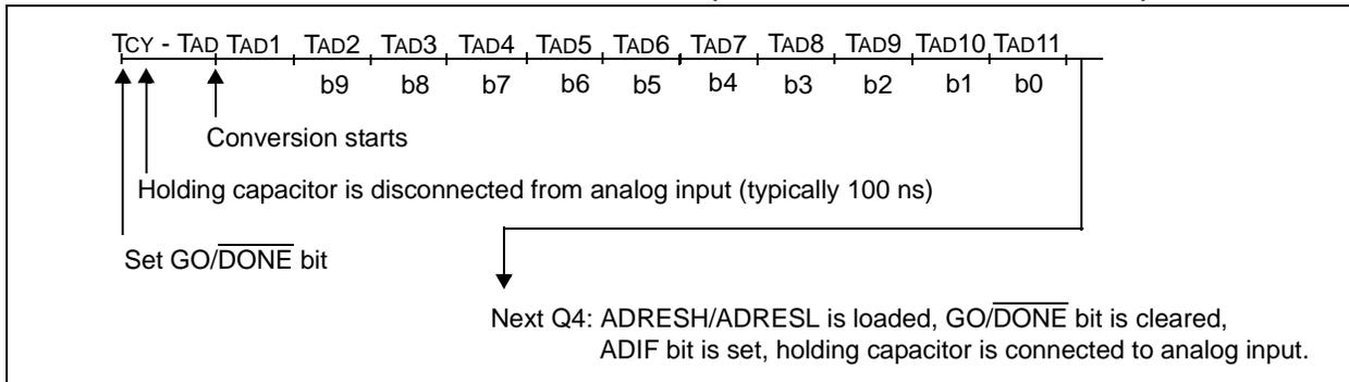
**FIGURE 17-4: A/D CONVERSION TAD CYCLES (ACQT2:ACQT0 = 010, TACQ = 4 TAD)**
