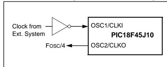
An external clock source may also be connected to the OSC1 pin in the HS mode, as shown in Figure 2-3. In this configuration, the divide-by-4 output on OSC2 is not available.
