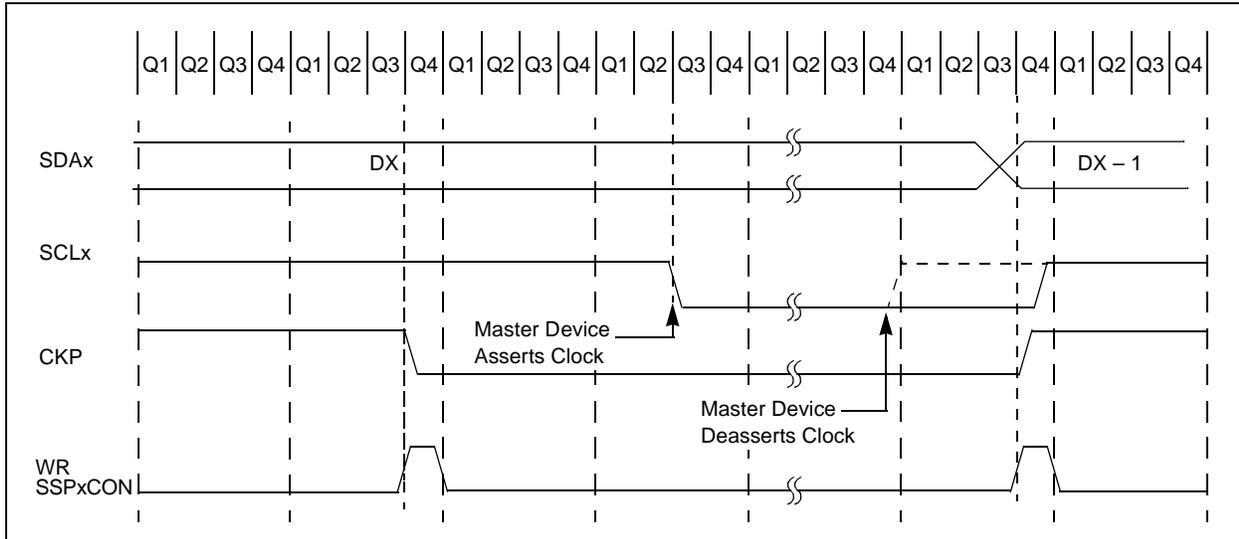
**FIGURE 15-13: I<sup>2</sup>C™ SLAVE MODE TIMING WITH SEN = 1 (RECEPTION, 7-BIT ADDRESSING)**
