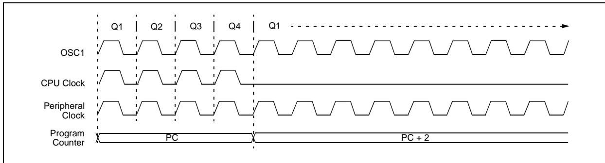
**FIGURE 3-7: TRANSITION TIMING FOR WAKE FROM IDLE TO RUN MODE**
