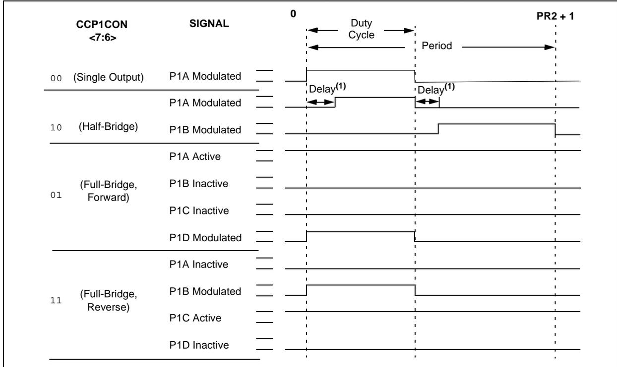
**FIGURE 14-3: PWM OUTPUT RELATIONSHIPS (ACTIVE-LOW STATE)**
