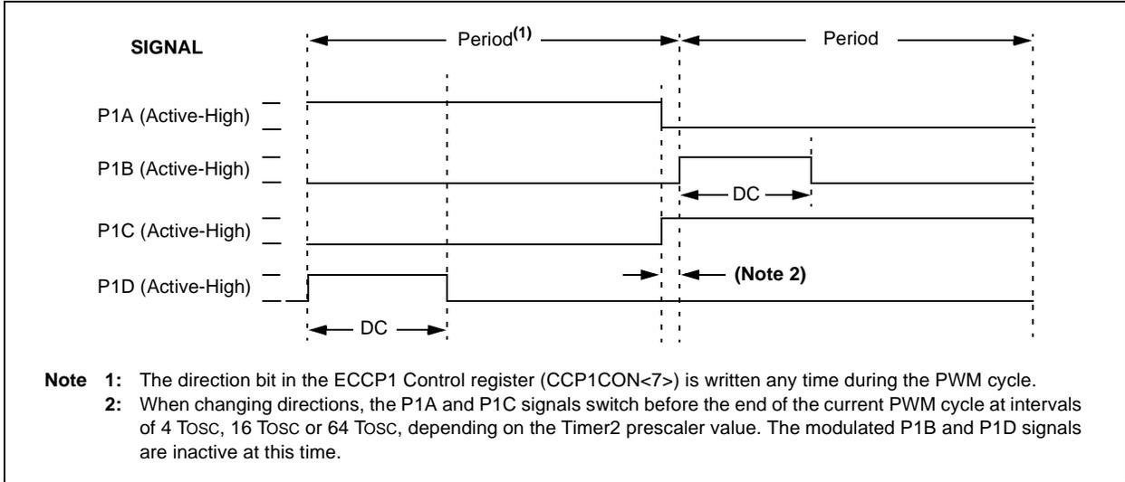
**FIGURE 14-9: PWM DIRECTION CHANGE AT NEAR 100% DUTY CYCLE**
