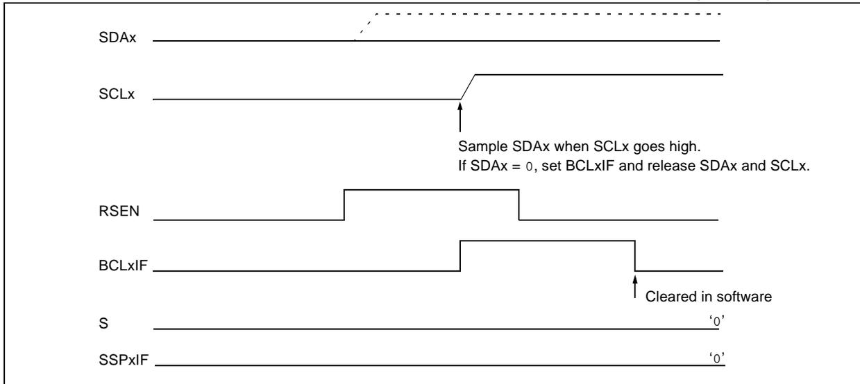
**FIGURE 15-30: BUS COLLISION DURING REPEATED START CONDITION (CASE 2)**
