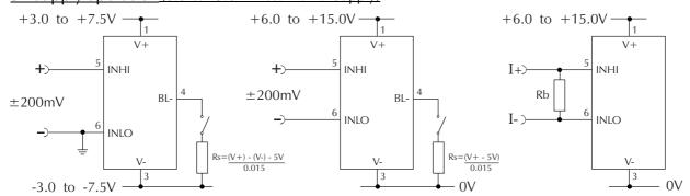
Measuring a single ended input voltage referenced to supply, i.e. the input voltage and the meter's power supply share the same 0V rail. Ensure solder link LCOM is open.
