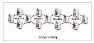
By the **MultiRing**<sup>TM</sup> Technology, user can enlarge the network campus just apply different Ring ID which is different with neighborhood to get unlimited Ring Coupling ability.
