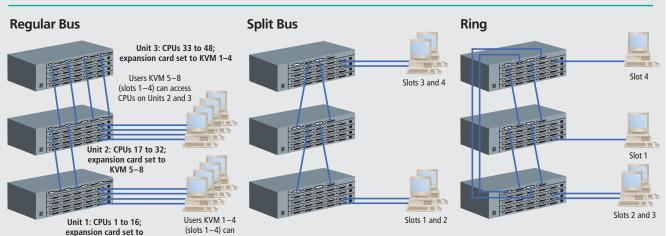
Because the control paths are carried on different connectors, you have maximum flexibility for designing your daisychain layout:
