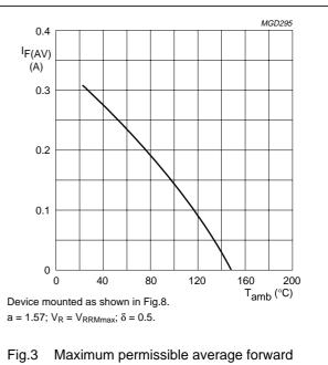
g.3 Maximum permissible average forward current as a function of ambient temperature (including losses due to reverse leakage).
