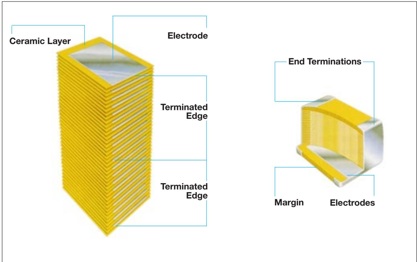
**Formulations** – Multilayer ceramic capacitors are available in both Class 1 and Class 2 formulations. Temperature compensating formulations are Class 1 and temperature stable and general application formulations are classified as Class 2.
