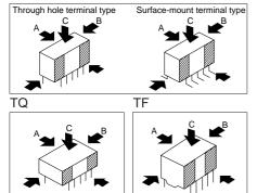
Please chuck the <u>minimize</u> portion. Avoid chucking the center of the relay. 2) TQ-SMD
