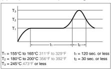
(2) Vapor phase soldering method
