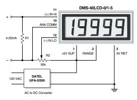
Figure 7. 4-to-20mA Current Loop Operation (5V-Powered Models)
