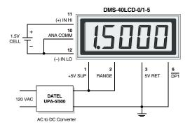
Figure 5. Floating Input Measurements (5V-Powered Models)
