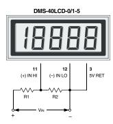
Figure 4. Input Attenuation Circuit
