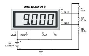
Figure 8. Power Supply Monitor (9V-Powered Models)
