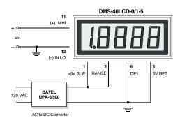
Figure 2. Single-Ended Input Configuration (5V-Powered Models)
