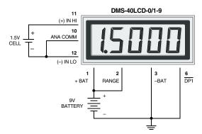
Figure 6. Floating Input Measurements (9V-Powered Models)
