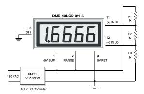
Figure 3. Differential Input Configuration (5V-Powered Models)
