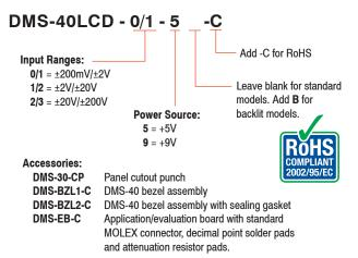
A panel-mount retaining clip is supplied with each model.
