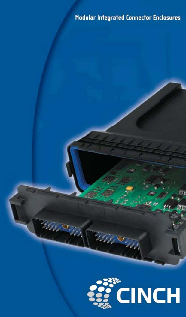
Cinch's Modular Integrated Connector Enclosures offer high quality sealed packaging solutions for rugged electronic control module applications. The Cinch 1.5mm SHS system is the base interconnect technology.
