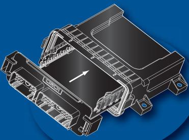
Assemble header/board into enclosure Push to lock and seal
