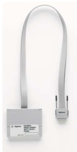
E5396A half-size Soft Touch connectorless probe
