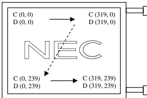
Figure1. DPSH= Low or Open (Normal scan)
