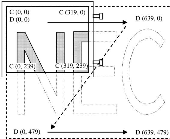
Figure1. DPSH= Low or Open (Normal scan)
