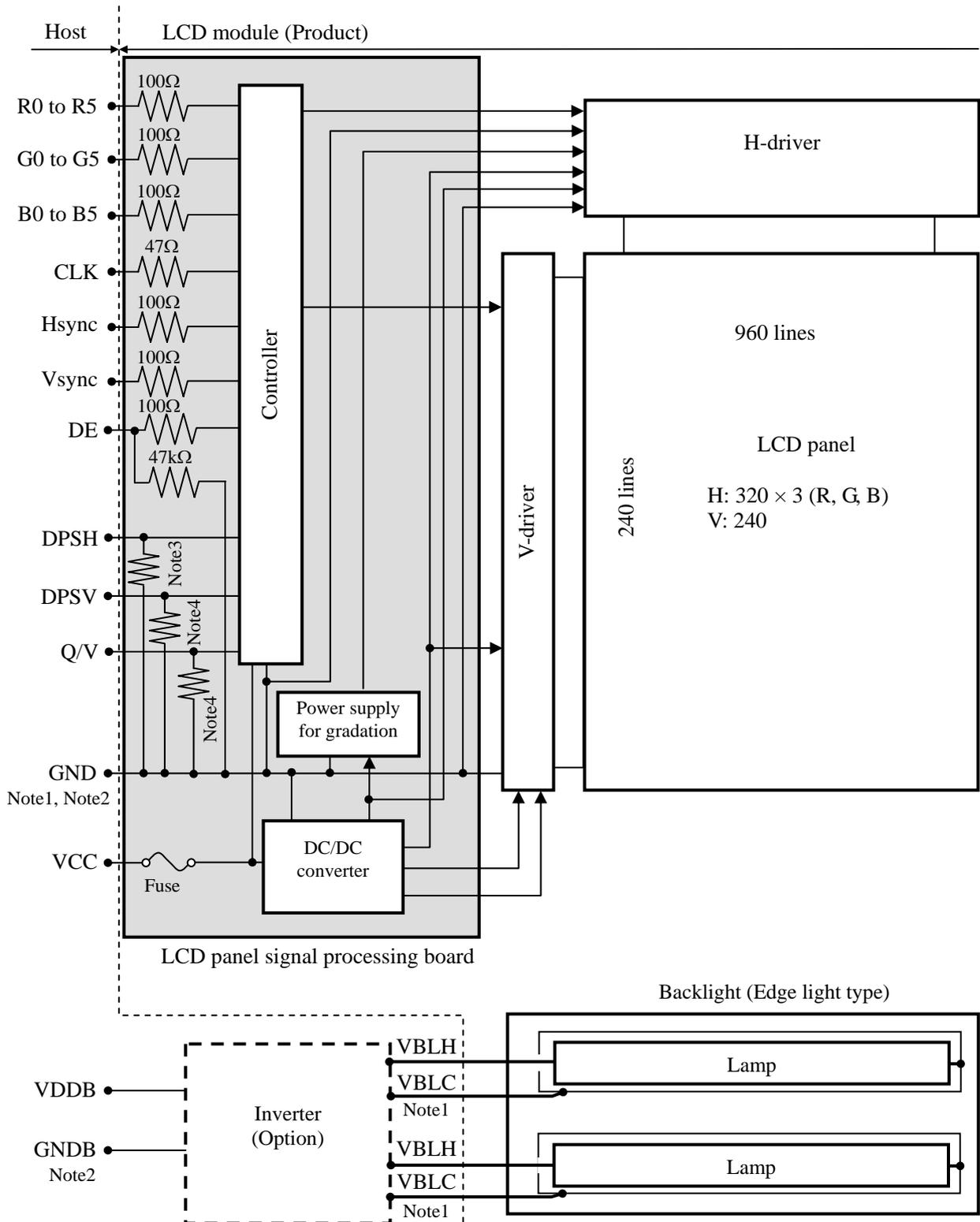
Note1: Relations between GND (Signal ground), shield plate and VBLC (Lamp low voltage terminal) in the LCD module are as follows.
