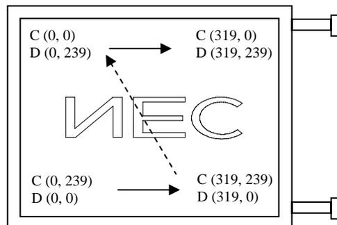
Figure3. DPSH= Low or Open (Normal scan)
