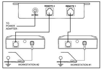
Figure 4. Wiring connection instructions for the <u>50516</u> / <u>50517</u> monitor control unit.
