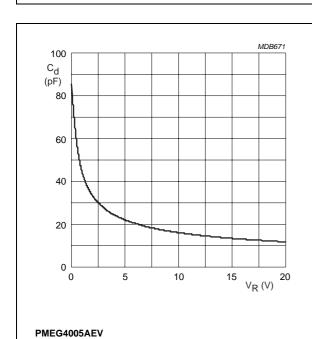
Fig.10 Diode capacitance as a function of reverse voltage; typical values.
