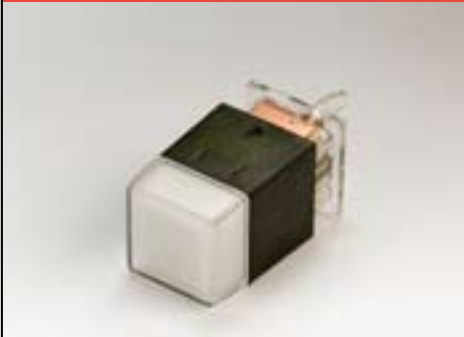
Illuminated pushbutton, front measurement 12.1 x 12.1 mm, plastic lens colourless transparent, PCP measurement 12.7 x 12.7 mm, 1 NO, IP40
