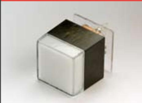
Illuminated pushbutton, front measurement 18.4 x 18.4 mm, plastic lens colourless transparent, PCP measurement 19.05 x 19.05 mm, 1 NO, IP40
