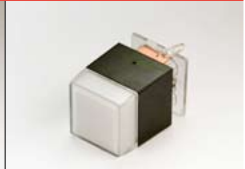
Illuminated pushbutton, front measurement 15.2 x 15.2 mm, plastic lens colourless transparent, PCP measurement 15.88 x 15.88 mm, 1 NO, IP40
