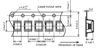
The packing directions of the chip coil in taping are unified with the in/out positions of the lead wire.
