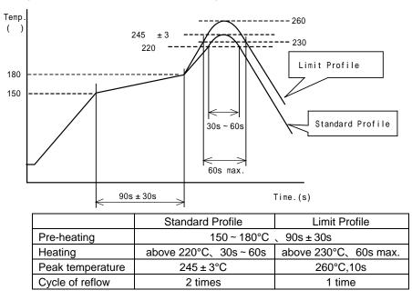
Soldering Profile for Eutectic solder
