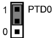
Figure 8-11: Accelerometer g-Select1 Jumper settings (J13)
