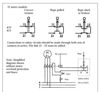
Notes: a) The terminal screws are M3.5 with rising cable clamps for ease of wiring.
