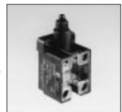
Terminal screws: M3.5 with rising cable clamps. Maximum screw tightening torque: 0.8Nm (8kg cm).
