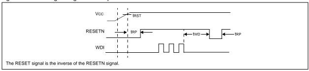
The watchdog is internally driven low during most (87.5%) of the watchdog timeout period (see two on page 5) and high for the rest of the watchdog timeout period. When pin WDI is left unconnected, this internal driver clears the watchdog timer every 1.4s. When WDI is tri-stated or is not connected, the maximum allowable leakage current is 10µA and the maximum allowable load capacitance is 200pF.
