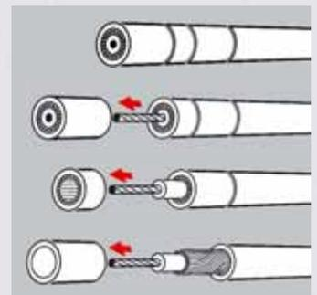
Dismantling of a Coax-cable in three steps
