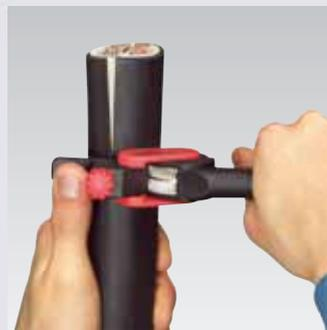
Turning the tool for circular cut
