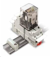
The 755 Magnetic Latching relay, with an 11 pin octal base, operates by using a pulsed input. A permanent magnet maintains the last position until a redirected second pulse moves the contacts back to the original state.
