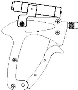
To turn flashlight on simply rotate the knob on the back of the flashlight Clockwise. To turn off the flashlight rotate the knob counterclockwise. Designed to be used with either 3" or 5" bits & sleeves. No adjustments necessary. Uses 1 AAA battery. To replace battery unscrew counterclockwise and remove knob, install new battery and replace knob.
