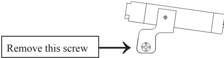
Remove the screw from the wire wrapping gun. This screw is no longer required (See sketch below).
