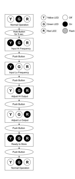
Figure 1: Q476 Calibration Flow Chart
