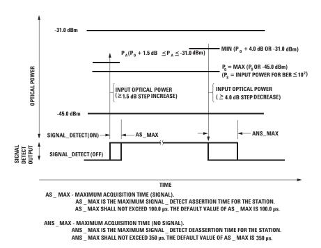
Figure 14. Signal Detect Thresholds and Timing.
