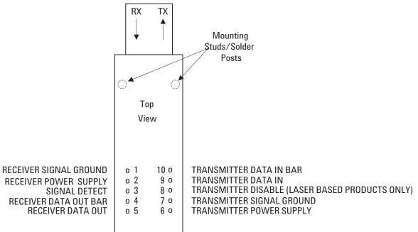
Figure 3. Pin Out Diagram.
