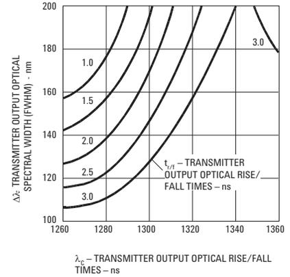
HFBR-5905 TRANSMITTER TEST RESULTS OF  $\lambda_c$ ,  $\Delta\lambda$ , AND  $t_{r/f}$  ARE CORRELATED AND COMPLY WITH THE ALLOWED SPECTRAL WIDTH AS A FUNCTION OF CENTER WAVELENGTH FOR VARIOUS RISE AND FALL TIMES.
