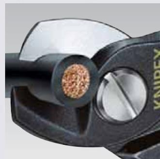
Cut effected with a Cable Shear: easy, clean cut without any deformation of the cable
