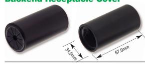
Provides environmental protection from dirt and debris and additional structural support to the back of receptacles. Particularly useful where the inside of enclosures are regularly accessed for maintenance. The slotted design enables a cable and RJ-45 to exit the cover and the threaded front end replaces the receptacle lock nut for panel mounting.
