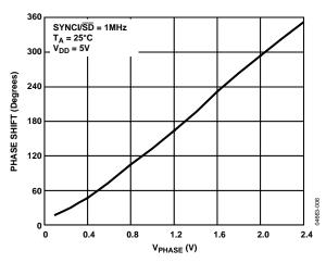
Figure 6. Clock Phase Shift vs. Phase Voltage
