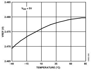
Figure 8. V<sub>REF</sub> vs. Temperature
