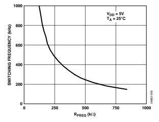
Figure 9. Switching Frequency vs. R<sub>FREQ</sub>
