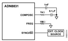
Figure 14. Synchronize to an External Clock
