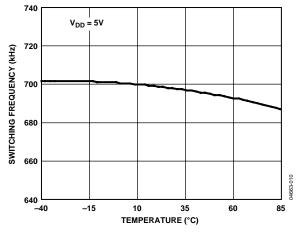
Figure 10. Switching Frequency vs. Temperature
