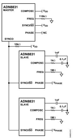
Figure 15. Multiple ADN8831 Devices Driven from a Master Clock
