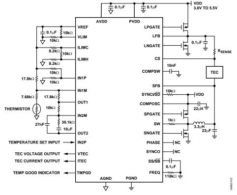
Figure 12. Typical Application Circuit 1
