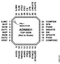
Figure 2. Pin Configuration
