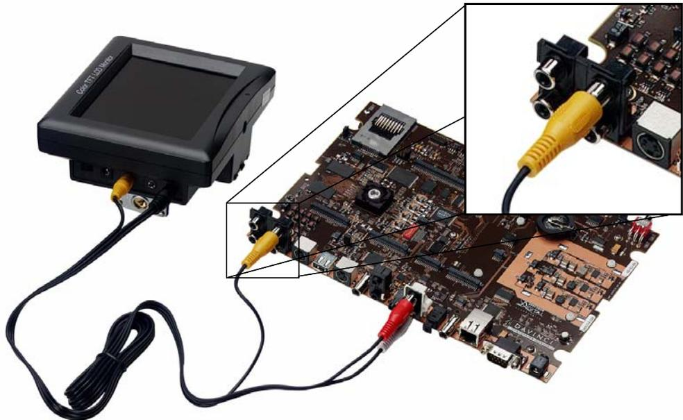
See Section A.2, *Changing the Video Input/Output Methods* for information about using S-Video or Component video.
