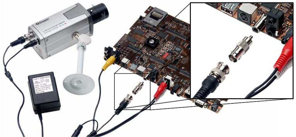
See Section A.2, *Changing the Video Input/Output Methods* for information about using S-Video or Component video.
