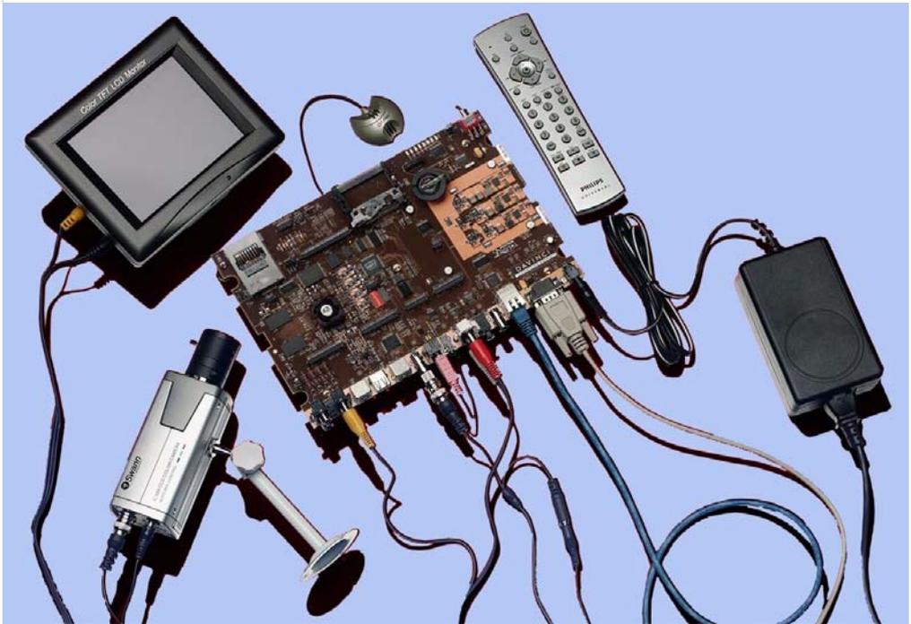
The intended audience is a user developing Linux-based software on the DM644x ARM core. The DVEVM does not expose the DSP core for software development, but rather treats it as a "black box" for running off-the-shelf codecs. Separate upgrade kits from Texas Instruments will provide tools and software for DSP development.
