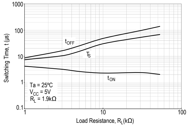
Figure 16. Switching Time vs. Load Resistance
