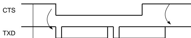
Figure 19-17. Transmitter Behavior when Operating with Hardware Handshaking
