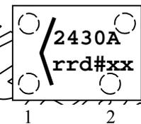
**Flip Chip, Top View with Laser Mark, Contacts Not Visible.**
