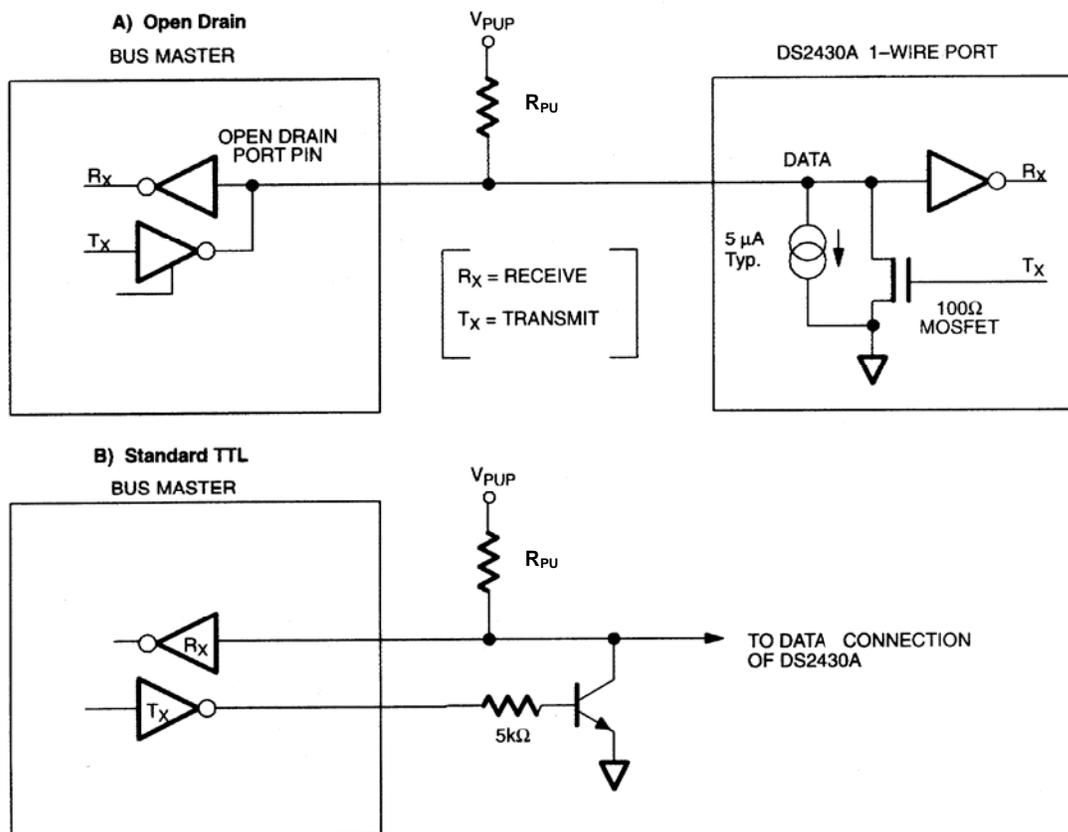
Note: Depending on the 1-Wire communication speed and the bus characteristics, the optimal pullup resistor value will be in the 1.5k $\Omega$  to 5k $\Omega$  range. To write to a single device, a 2.2k $\Omega$  resistor and  $V_{PUP}$  of at least 4.0V is sufficient. For writing multiple DS2430As simultaneously or operation at low  $V_{PUP}$ , the resistor should be bypassed by a low-impedance pullup to  $V_{PUP}$  while the device copies the scratchpad to EEPROM.
