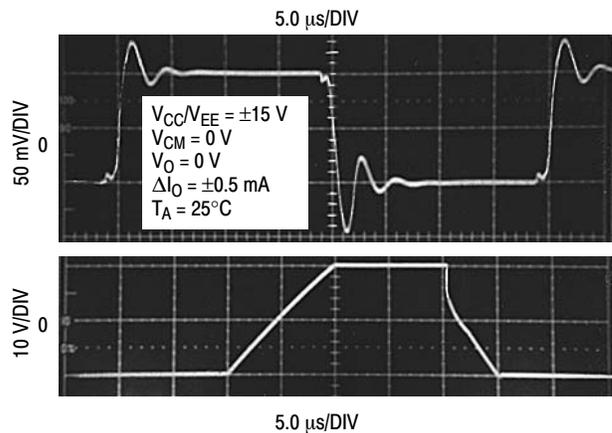
Figure 7. Small and Large Signal Transient Response
