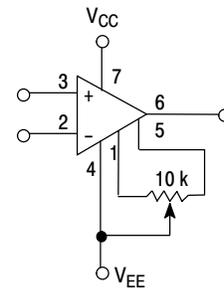
Offset Nulling range is approximately  $\pm 80 \text{ mV}$  with a 10 k potentiometer, MC33171 only.
