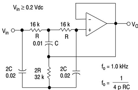
Figure 14. Active High-Q Notch Filter
