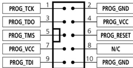
Figure 4.9.1 - Atmel 10-way IDC Header (J8) viewed from above
