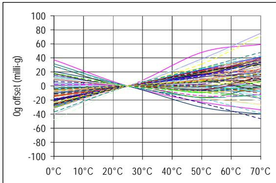
Graph 11. Examples of A\_OUTX 0g offset vs. temperature
