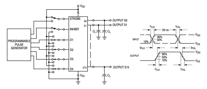
Figure 3. Switching Time Test Circuit and Waveforms
