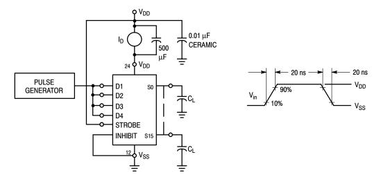
Figure 2. Dynamic Power Dissipation Test Circuit and Waveform
