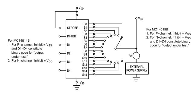
Figure 1. Drain Characteristics Test Circuit
