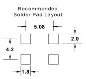
Note: XPRESSO HCMOS XOs are designed to fit or industry standard, 4 pad, layouts.
