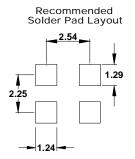
Note: XPRESSO HCMOS XOs are designed to fit on industry standard, 4 pad, layouts.
