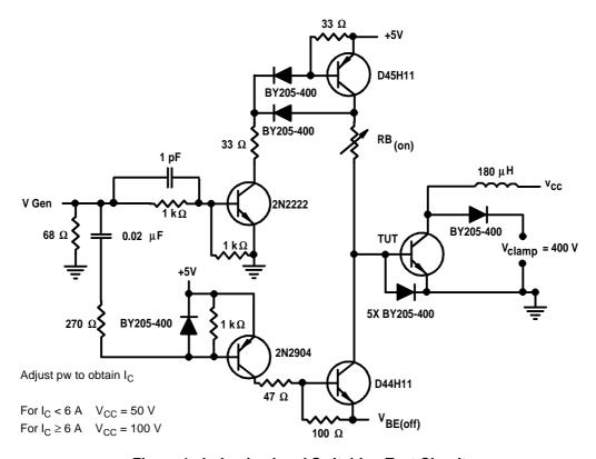
Figure 1. Inductive-Load Switching Test Circuit
