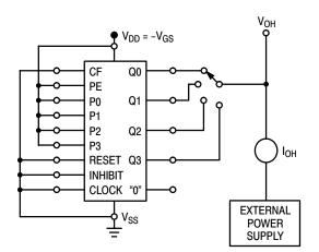
Figure 1. Typical Output Source Characteristics Test Circuit
