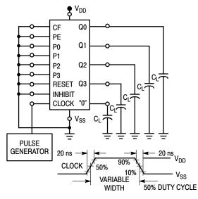
Figure 3. Power Dissipation
