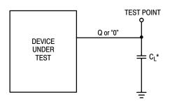
\* Includes all probe and jig capacitance.
