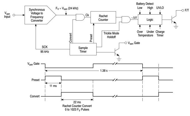
Figure 10. Negative Slope Voltage Detector
