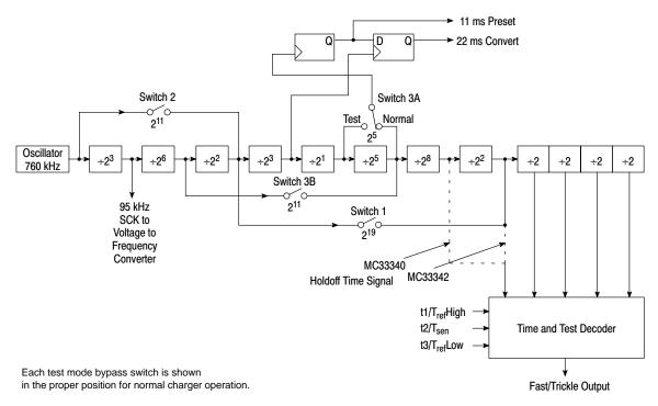
Figure 11. Timer Functional Block Diagram
