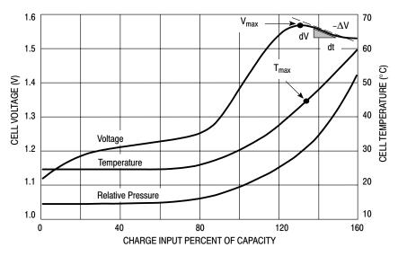
Figure 9. Typical Charge Characteristics for NiCd and NiMh Batteries
