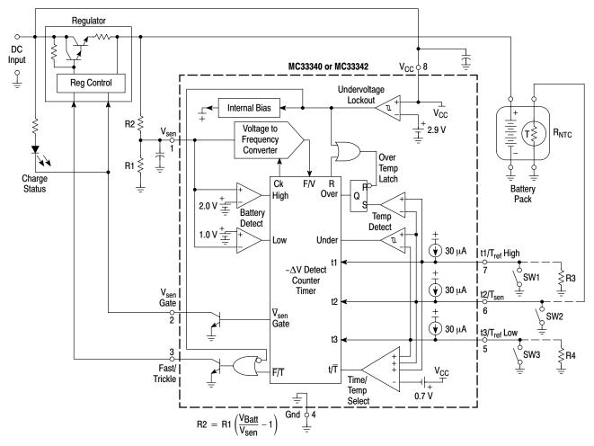
Figure 8. Typical Battery Charging Application
