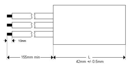
AMPOHM Delta Suppressors are designed for the interference suppression of small motors, business machines and a wide range of domestic appliances in the broadcast band from 20Khz to 3Mhz.
