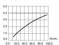
FIG.3 RELATIVE LUMINOUS INTENSITY VS. FORWARD CURRENT.
