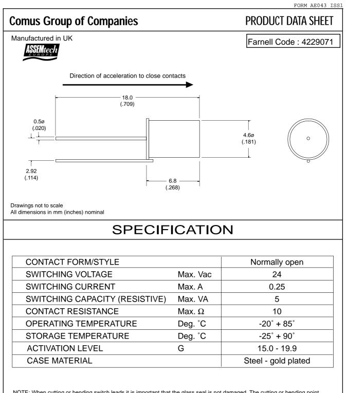
NOTE: When cutting or bending switch leads it is important that the glass seal is not damaged. The cutting or bending point should be no closer than 3mm (.118) to the glass to metal seal and the lead should be supported between the cutting or bending point and the glass to metal seal.
