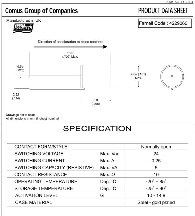
NOTE: When cutting or bending switch leads it is important that the glass seal is not damaged. The cutting or bending point should be no closer than 3mm (.118) to the glass to metal seal and the lead should be supported between the cutting or bending point and the glass to metal seal.
