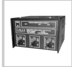
The BPS5000 provides three fully stabilised and smoothed variable DC power sources. Maximum versatility is achieved by making each output isolated from the other so that they may be interconnected to provide plus and minus rails or added together for higher voltages.
