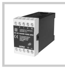
The 41000 Series range of power supplies are designed for quick and trouble-free installation onto 35mm profile DIN rails. With outputs ranging from 5V to 24V and maximum current capabilities from 100mA to 500mA, these units are ideal for most instrumentation and control systems.
