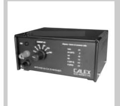
The BPS1000 constant current nickel cadmium battery charger is designed for quick charging, overnight charging or float (trickle) charging of a single cell or up to a maximum of 7 cells in series – as in a battery pack.
