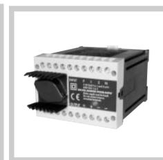
The 42000 Series DIN rail mounting power supplies are supplied ready for connection. The unit has only to be snapped on to the 35mm profile rail (DIN 46277-3) and connected to the clearly marked terminal screws. A status LED indicates power OK.
