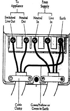
For bottom cable entry use the cable clamps provided to grip the cable outer and provide strain relief.
