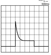
8-(2). Electrical life test (Halogen lamp load) Sample: CM1aF-R-12V, 6pcs. Load: 20A 13.5V DC Switching frequency: (ON:OFF = 1s:14s) Ambient temperature: Room temperature
