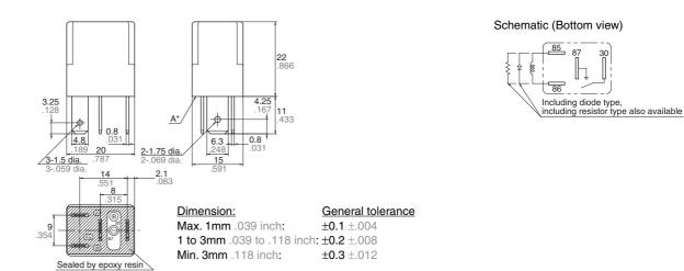
\* Intervals between terminals is measured at A surface level.
