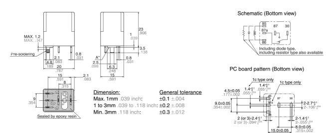
\* Dimensions (thickness and width) of terminal specified in this catalog is measured before pre-soldering. Intervals between terminals is measured at A surface level.
