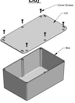
Purchased assembly includes box, lid and 4 cover screws. Box and lid are made from Diecast Aluminum Alloy (alloy type 360.1).
