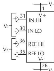
Measuring the ratio of two voltages.
